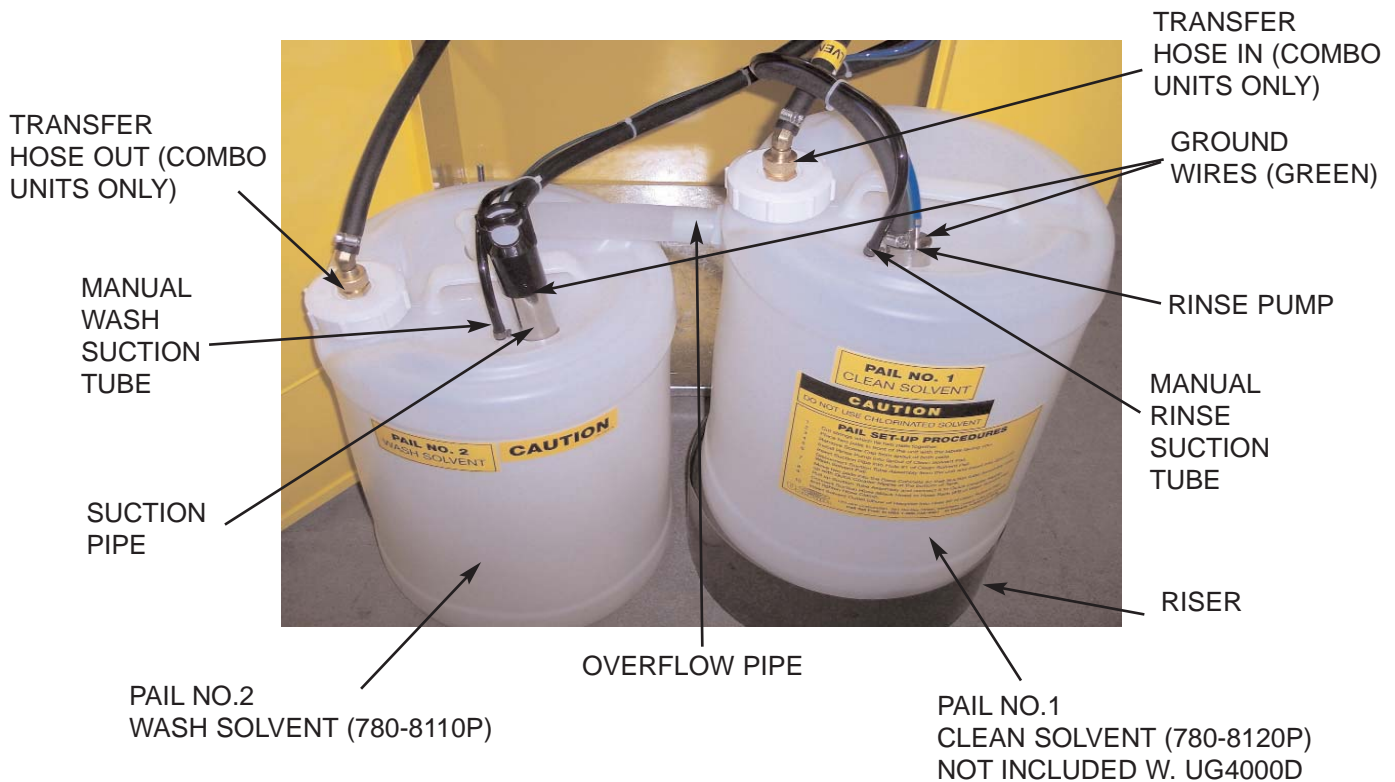
SOLVENT PAIL SETUP - PLASTIC PAILS
